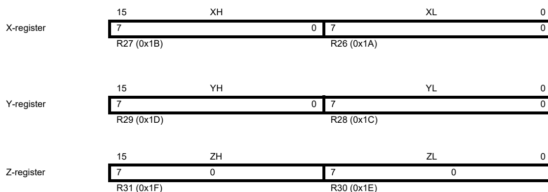
Figure 7-3. The X-, Y- and Z-Registers
